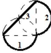
Fig. E2. Sketch to deduce the view factor F_{12} between two long hemicylinders (1) and (2).
